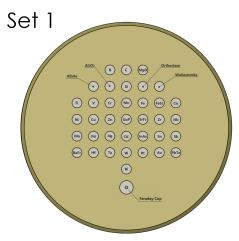
37 standards covering 42 elements plus Faraday cup. 32mm diameter x 5mm deep brass block. Supplied with data sheet.
